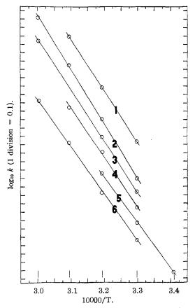
Fig. 3.—Plots which gave the activation energies, E, in Table I. The vertical lines in the plot along the abscissas are at values of 1/T at 60, 50, 40, 30 and 20° from left to right, respectively. The numbered lines represent the data for the compound with the same number in Table I.
