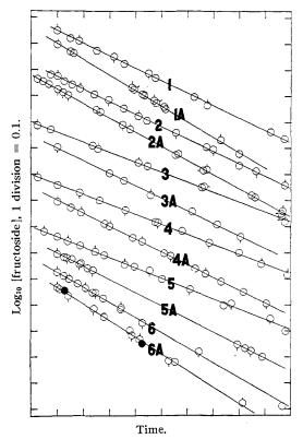
Fig. 2.—Typical plots of data which gave the fraction of fructoside hydrolyzed per minute. The numbered unlettered lines represent data at the highest temperature and the A lines at the lowest temperature listed in Table I for the compound with the same number. One division on the abscissas represents in minutes for line 1, 20; 1A, 400; 2, 10; 2A, 1000; 3, 5; 3A, 400; 4, 5; 4A, 100; 5, 10; 5A, 200; 6, 20 and 6A, 1000.
